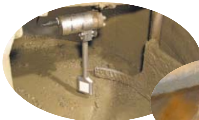
The Hydro-Probe Orbiter with The Hydro-Control V is the perfect combination for controlling the water in your mixer.
